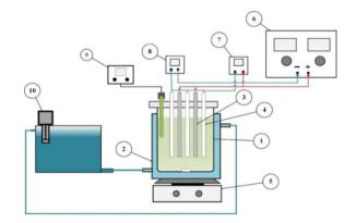
**Figure 1**. The electrochemical system: 1) cell body, 2) jacket, 3) iron anode, 4) stainless steel cathode, 5) magnetic stirrer, 6) power supply, 7) voltmeter 8) Ammeter,9) pH-meter,10) water bath circulator.
