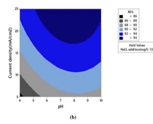
Figure 2. The combined effects of current density and solution pH on the COD removal efficiency at constant addition of NaCl (1.5 g/l): (a) 3D surface plot,(b) contour plot.
