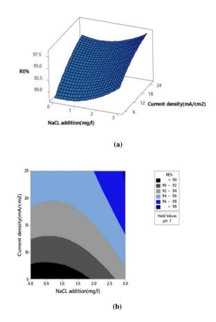
**Figure 4.** The combined effects of current density and addition of NaCl on the COD removal efficiency at constant solution pH=7(a) 3D surface plot,(b) contour plot.
