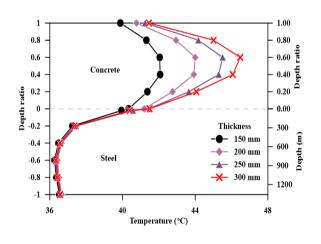
Figure 23. Thickness effect on temperature gradient at 0:00 hr on (24-July).
