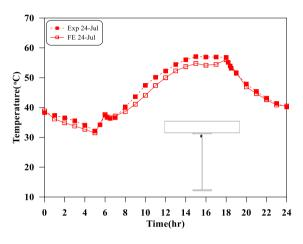
Figure 15. Hourly experimental recorded and FE expected temperatures at the TS9 thermocouple of the composite segment.
