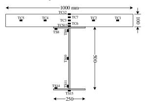
Figure 1. Dimensions and thermocouples locations.
