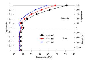
Figure 30. Effect of wind speed on the temperature gradient in the composite section on a summer day (24-July @ 14:00).
