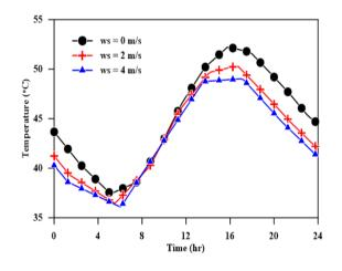
Figure 29. Effect of wind speed on the temperature variation of the bottom surface concrete slab on a summer day (24 July).
