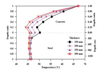
Figure 22. Thickness effect on temperature gradient at noon hr on (24-July).
