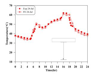
Figure 16. Hourly experimental recorded and FE expected temperatures at the TS11 thermocouple of the composite segment.
