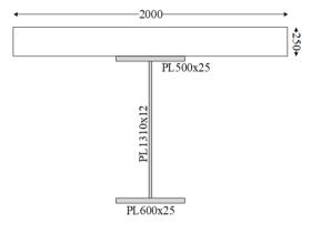
Figure 17. Dimensions of the bridge section.
