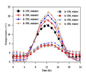
Figure 20. Effect of thickness on the variance between the upper surface temperature and the temperature at a depth of 60% of the slab thickness.
