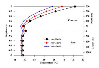
**Figure 25.** Effect of asphalt layer thickness on the temperature distribution with a depth of the composite bridge at hr=15:00.
