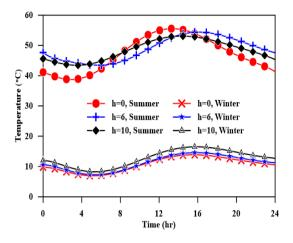
Figure 27. Effect of an asphalt layer on the maximum and minimum average temperature of the composite bridge.
