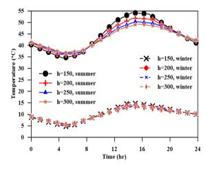
Figure 19. Effect of slab thickness on the bottom surface temperature in 24-July and 15-January.
