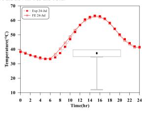
Figure 13. Hourly experimental recorded and FE expected temperatures at TC3 thermocouple of a composite segment.
