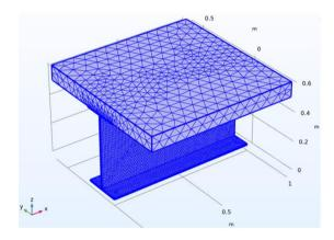
Figure 11. The mesh of the composite bridge segment.
