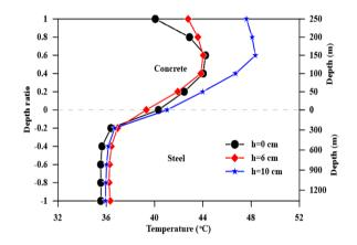
**Figure 26.** Effect of asphalt layer thickness on temperature distribution with the depth of the composite bridge at hr=1:00.
