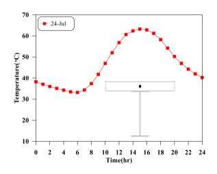
Figure 7. Temperature change in (TC3) thermocouple during a Sunny day.
