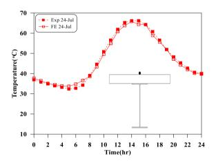
Figure 14. Hourly experimental recorded and FE expected temperatures at TC12 thermocouple of a composite segment.
