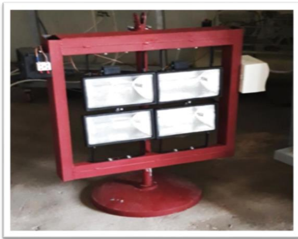
Figure 3. Heat source or solar simulator
