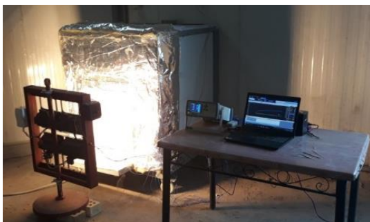
Figure.6. Install sensors on both sides of the wall and in middle of the room
