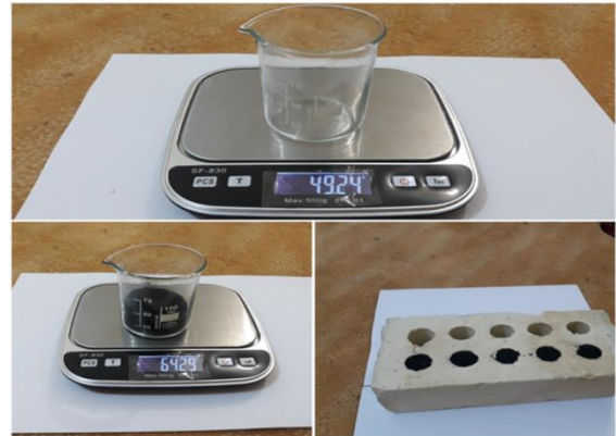
Figure8. Put 15g of scrap tire powder into one hole
