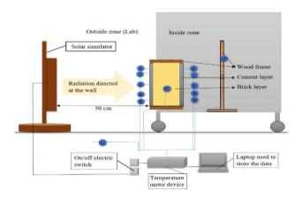
**Figure 5.** Schematic of the experimental and the distribution of the sensor.
