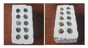
Figure 4. Perforated brick filled with PCM capsule.
