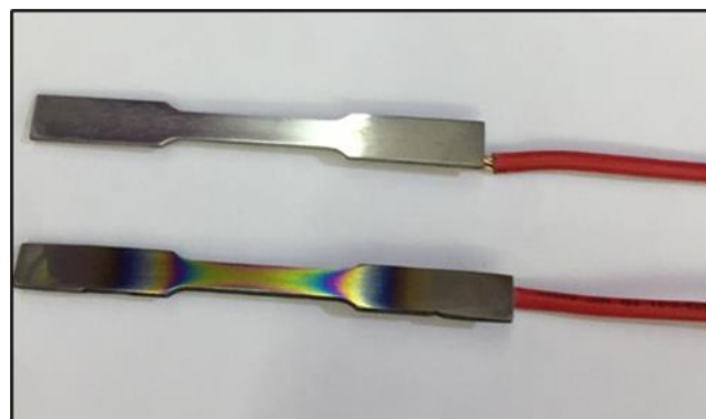
Figure 2. Coated and uncoated work substrate before covering
