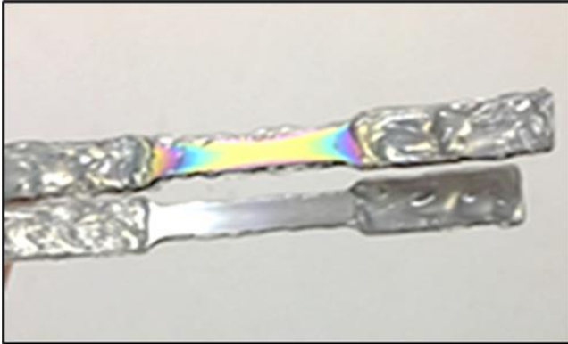
Figure 3. Partially covered tensile test specimens by epoxy resin
