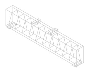
Figure 1. Traditional closed and spiral stirrups of beam B1 and B2
