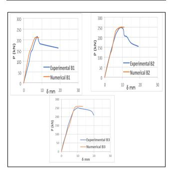
Figure 4. The load-defection of the beam with different pattern stirrups
