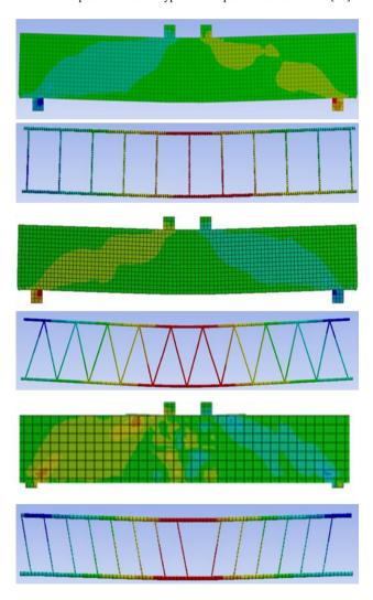
Figure 5. Shear patterns in concrete and steel of beams B1, B2 and B3 at failure.
