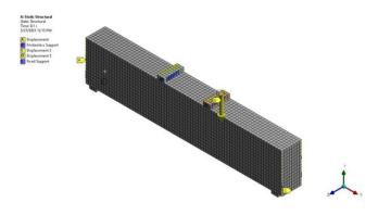
Figure 2. Quadrilateral mesh of concrete
