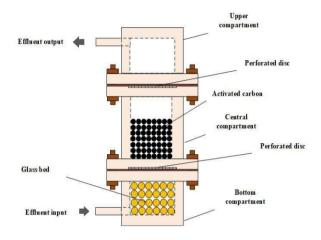
Figure 2 Schematic diagram of the chemical reactor
