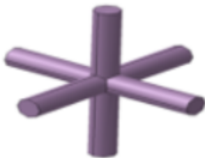
Figure 3. 3D Circular unit cell element
