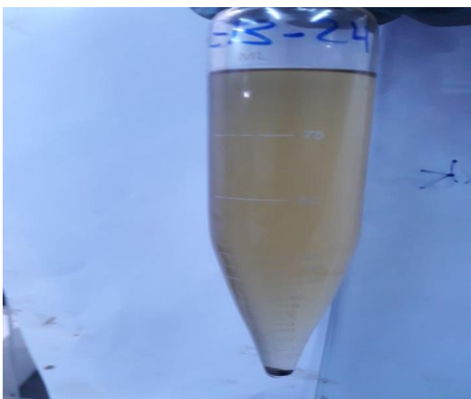
Figure 7. Shows the deposition of asphalt at the end of the tube.
