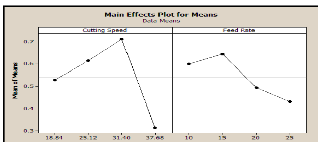
Figure 11. The influence of feed rate and cutting speed on surface roughness for down-cut milling on fluid machines
