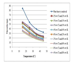
Figure 9. Effect of toluene & kerosene weight fraction on the viscosity of Missan heavy crude oil.
