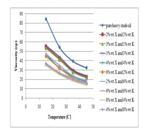
Figure 11. Effect of xylene & kerosene weight fraction on viscothe sity of Missan viscous crude oil.
