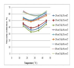
Figure 4. Effect of naphtha & toluene weight fraction on viscosity reduction of Missan crude oil.
