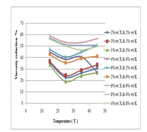
Figure 12. Effect of xylene & kerosene weight fraction on viscosity reduction of Missan heavy crude oil.
