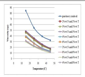
Figure 3. Effect of naphtha & toluene weight fraction on the viscosity of Missan crude oil.
