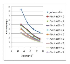
Figure 5. Effect of naphtha & xylene weight fraction on the viscosity of Missan viscous oil.
