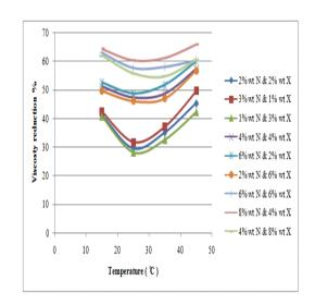
Figure 6. Effect of naphtha & xylene weight fraction on viscosity reduction of Missan heavy crude.
