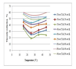
Figure 10. Effect of toluene & kerosene weight fraction on viscosity reduction of Missan crude oil.
