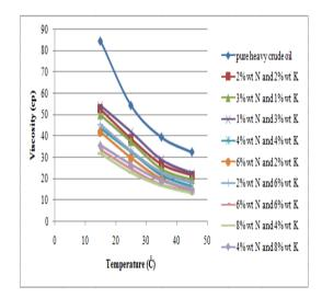
Figure 7. Effect of naphtha & kerosene weight fraction on the viscosity of Missan viscous crude oil
