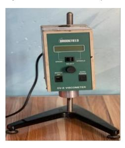
Figure 1. DV-EViscometer used for viscosity measurements.
