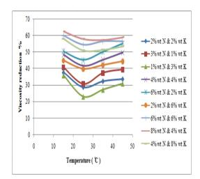
Figure 8. Effect of naphtha & kerosene weight fraction on viscosity reduction of Missan heavy oil.
