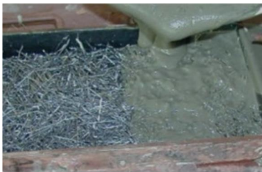
Figure 1. Casting procedure of SIFCON
