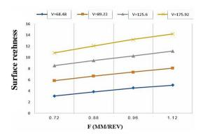
Figure 5. Show the comparison between surface roughness and feed rate for steel 45 at different cutting speeds
