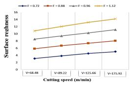
Figure 9. Depicts a comparison of surface roughness and cutting speed for (Steel Y8) at various feed rates
