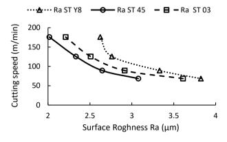
Figure 10. Compares the cutting speed and SR for three metals (Steel 03, 45 and Y8)
