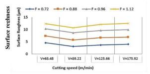
Figure 8. Compares the Ra and speed of cut for Steel 45 at various feed rates
