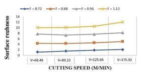
Figure 7. Compares Ra and cutting speed for steel 03 at different feed rates
