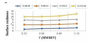
Figure 4. Show the comparison between surface roughness and feed rate for steel 03 at different cutting speeds
