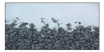
Figure 1. Cementitious grout during the process of penetrating the voids of a porous asphalt skeleton [24]
