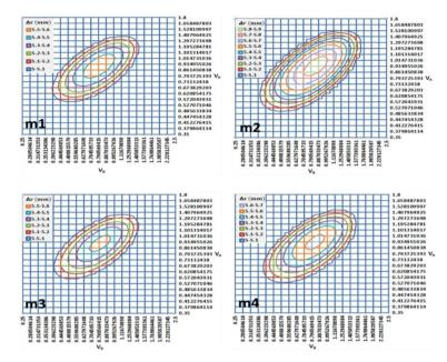
Fig. 5: A two-dimensional surface plot of the beam diameter relative to both voltage percentages  $(V_A)$  and  $(V_B)$  of the electrostatic lenses (m1, m2, m3 and m4) in the acceleration mode.
