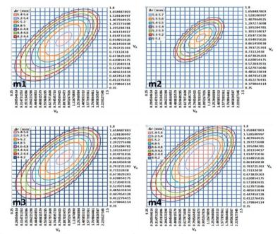
Fig. 6: A two-dimensional surface plot of the beam diameter relative to both voltage percentages  $(V_A)$  and  $(V_B)$  of the electrostatic lenses (m1, m2, m3 and m4) the deceleration mode.
