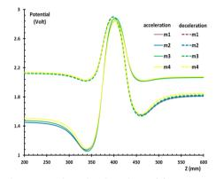
Fig.(2): The axial potential distribution of four electrostatic lenses (m1, m2, m3, and m4) in acceleration and deceleration
