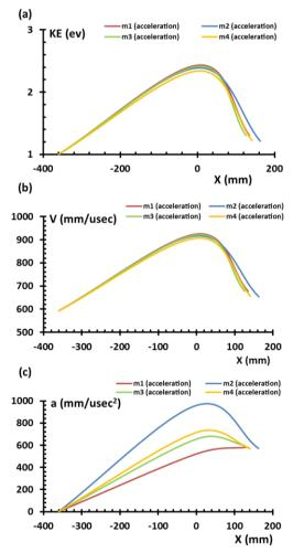
Fig. 3: Comparison of (a) the kinetic energy, (b) the velocity, and (c) the acceleration of the charged particles at the cross over point relative to the main axis in the acceleration mode of the electrostatic lenses (m1, m2, m3 and m4).
