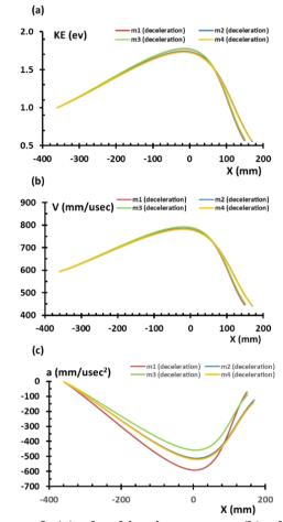
Fig. 4: Comparison of (a) the kinetic energy, (b) the velocity, and (c) the acceleration of the charged particles at the cross over point relative to the main axis in the deceleration mode of the electrostatic lenses (m1, m2, m3 and m4).
