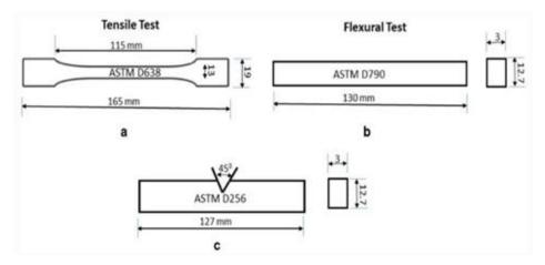
Figure 4 (a) ASTM D638 standard for tensile samples. (b) ASTM D790 standard for flexural samples. (c) ASTM D256 standard for impact charpy samples.
