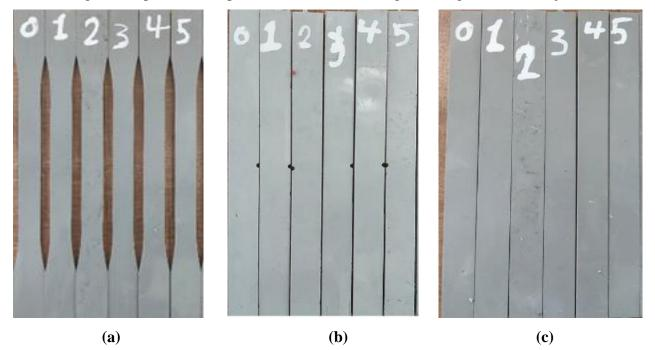
Figure 3 (a) Tensile test samples, (b) Impact test samples, (c) Flexural test samples.
