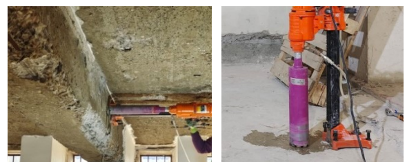
a) Core B at beam b) Core D at slab Fig. 10 Cores sampling.
