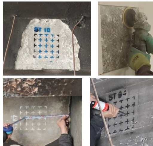
Fig. 6 Arrangements for hammer test at each station.
