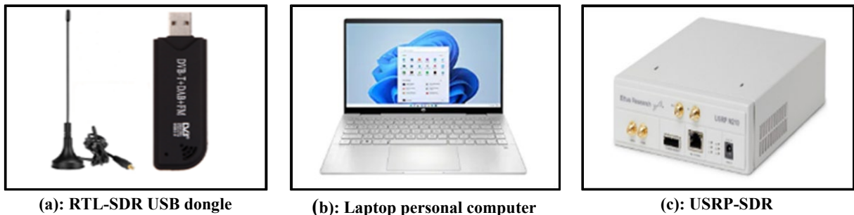
Figure 2: The essential adopted SDR hardware components for MSKU3-based CSS, (a): RTL-SDR USB dongle, (b): Laptop personal computer, (c): USRP-SDR
