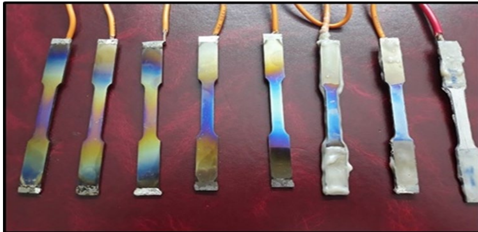
Figure 5: The tensile specimen after the coating process
