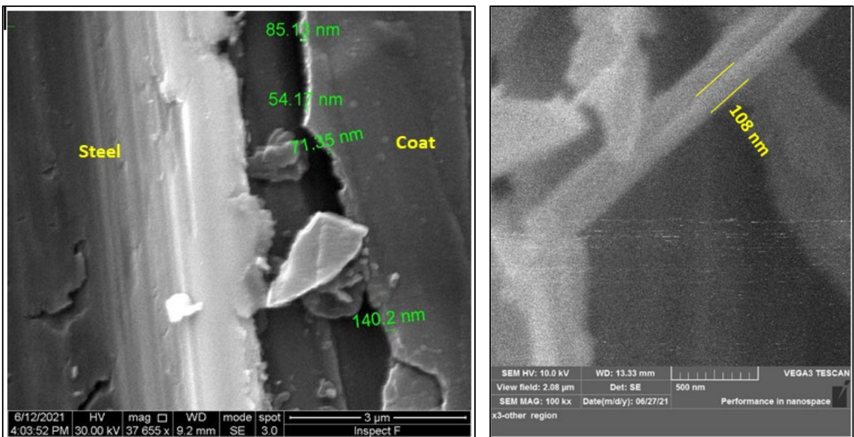
Figure 8: SEM image of Ti thin layer coating at a - 37kx b – 100kx
