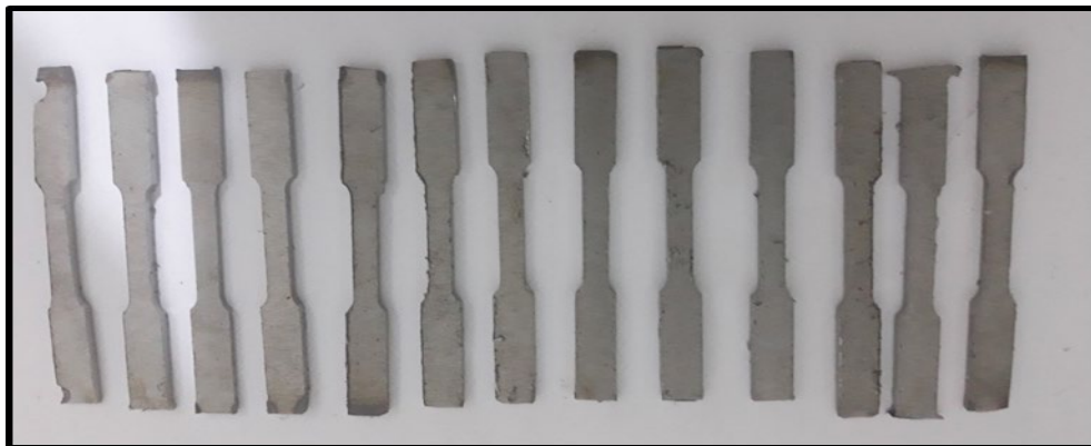
Figure 3: The manufactured AISI 1018 steel specimens according to ASTM-E8
