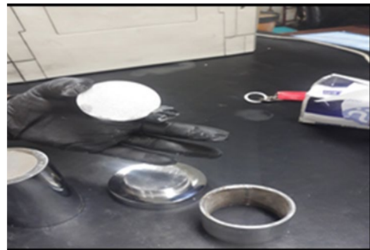
Figure 2: Aluminium target after extracted from S.S. dye mold
