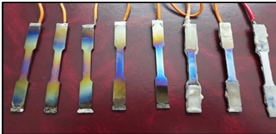
Figure 5: The tensile specimen after the coating process
