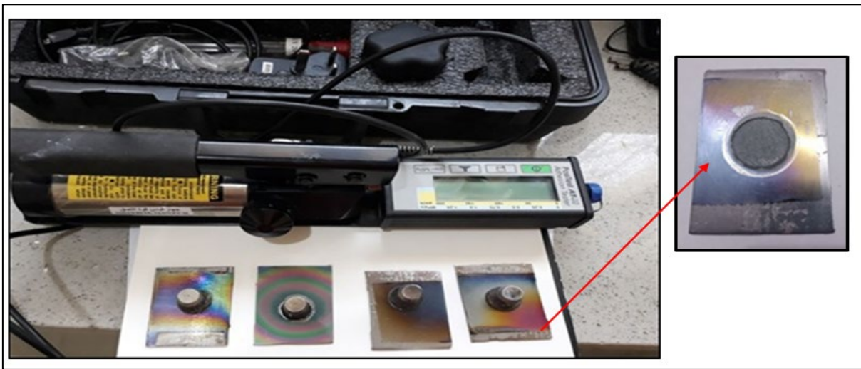
Figure 7: Adhesive strength examination device
