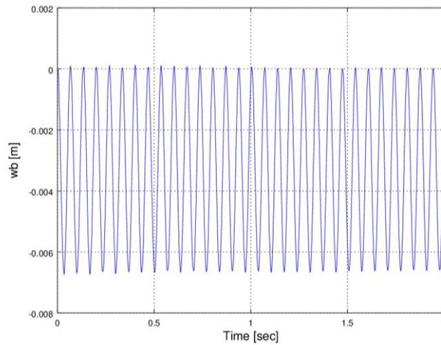
**Fig. 6 b** Dynamic mid-span  $w_b(t)$  of the numerical simply supported beam of 6 m length with  $K_n = 0.5 \times 10^8$  N/m and  $K_s = 10^8$  N/m due to a uniform step 1 kN load, for a period of 2 seconds
