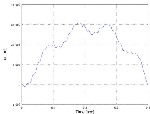
**Fig. 3 a** The variation of  $u_a(t)$  near the roller support of Shen *et al.*'s (2011) example corresponding to a 1 Newton force crossing the beam at 10 m/sec as computed by the present model
