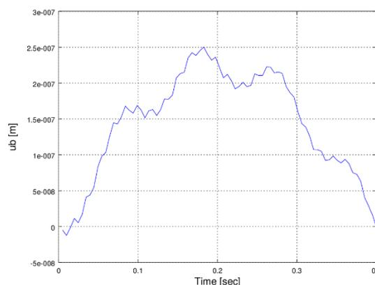
**Fig. 3 b** The variation of  $u_b(t)$  near the roller support of Shen *et al.*'s (2011) example corresponding to a 1 Newton force crossing the beam at 10 m/sec as computed by the present model
