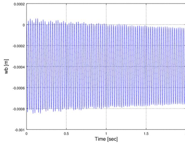
**Fig. 7 b** Dynamic mid-span  $w_b(t)$  of the numerical simply supported beam of 5 m length the lower layer of which was fixed at both ends due to a uniform step 1 kN load, for a period of 2 seconds
