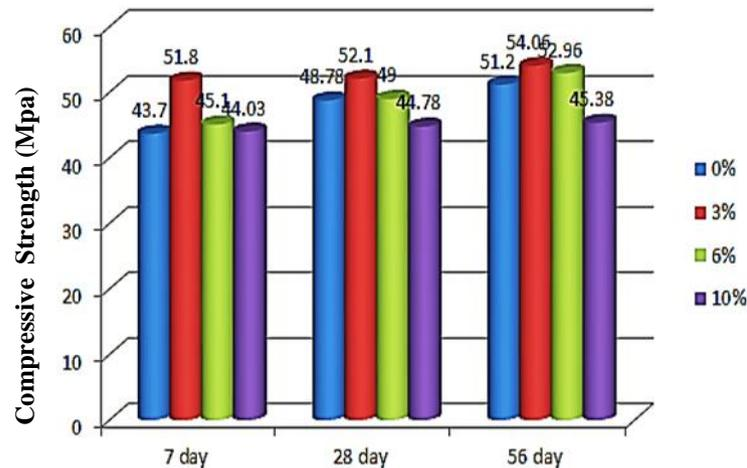
**Fig. 3 Shows the relationship between compressive strength, age, and the percentage of fibers in SIFCON.**
