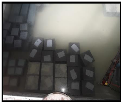
Fig.4.4 Curing the Cubes
