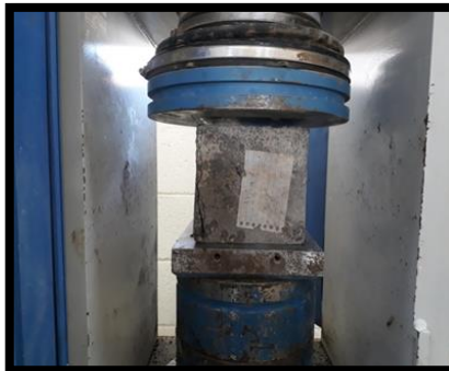
Fig.4.5 Compressive strength device
