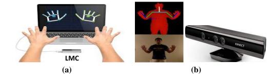
Figure 5 (a) Leap motion controller (LMC), (b) Microsoft Kinect (MSK) [21]. 4. Methods for Sign Identification Systems
