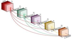
Figure 14. DenseNet architecture with five layers [52].
