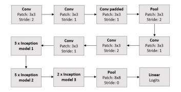
Figure 6. The underlying architecture of Inception v3.
