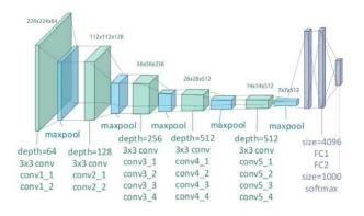
Figure 8. [31] VGG 19 network architecture.
