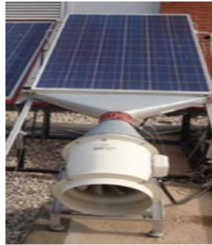
Figure 3. Shows the forced convection air cooling [19].
