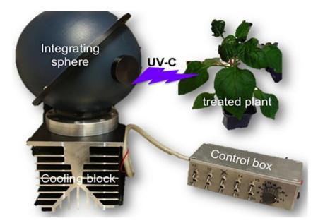
Fig. 1: The device used to provide the plants with the ultra violet ray. The internal part contains 15 UV-C lamps as a circular shape. The 5 cm-radius spherical window is removed and the rays is directed to the leaves straightforward.
