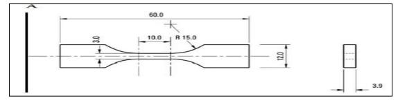
Figure 1: Sample for measurement of tensile strength
