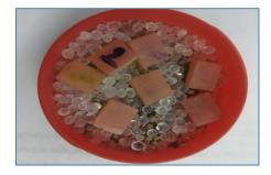
Figure (2) Acrylic specimens were dried by silica gel
