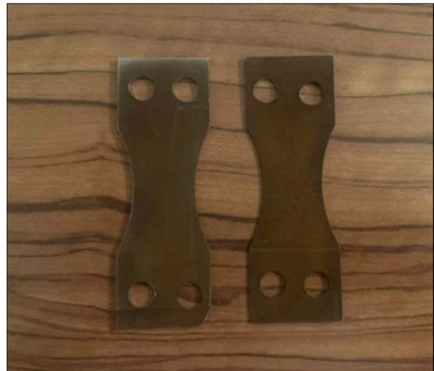
Figure 2: The St.52 blades of the steam turbine, after cutting
