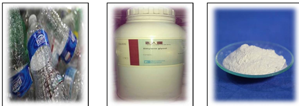
Figure 2: Materials used in this work. (a) The unsaturated waste plastic bottles (PET), (b) Ethylene Glycol (EG.), (c) Magnesium Oxide (Nano catalyst)
