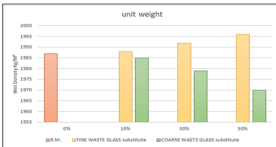
Figure 5: Effect of glass substitution percentages on unit weight
