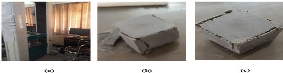
Figure 3: Computer-controlled electronic universal machine by Laree technology co., ltd (a) and cubes specimen shape at failure (b, c)
