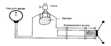
Figure 2 Mercury injection pump[21]
