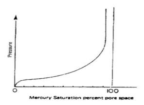
Figure 3 Porosity through mercury injection[21]
