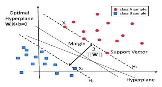
Figure 7 Classification of data by support vector machine[24]
