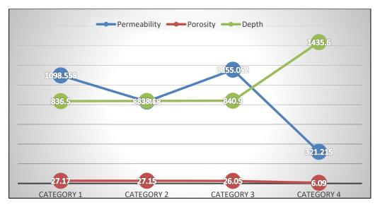
Figure 9 Comparison chart between porosity, permeability, and depth
