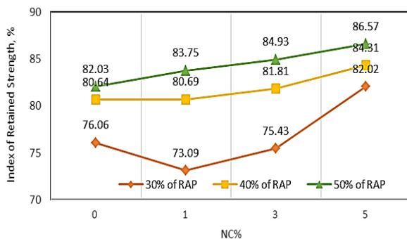
Figure 5: The Impact of Nono-clay Content on the Index of Retained Strength
