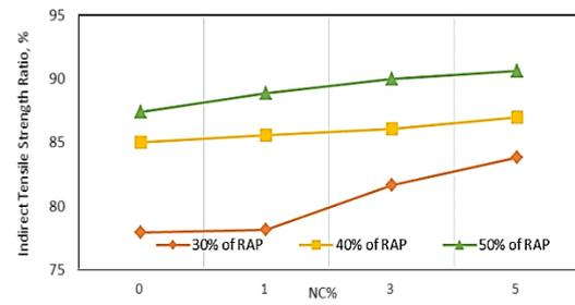
**Figure 8:** Influence of Nono-clay percent on Indirect Tensile Strength Ratio.
