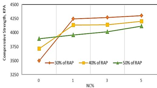
**Figure 3:** The Impact of Nano-clay Content on Compressive Strength for the Unconditioned Sample
