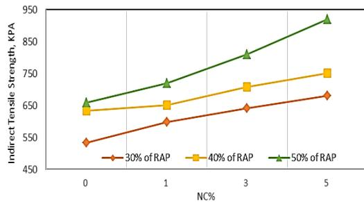
**Figure 7:** Influence of the amount of Nanocly on the Indirect Tensile Strength for the Conditioned Sample.
