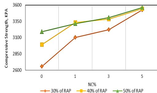
**Figure 4:** The Impact of Nano-clay Quantity on Compressive Strength for the Conditioned Sample.
