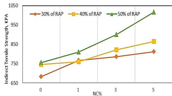
Figure 6: Influence of Nono-clay percent on the Indirect Tensile Strength for the Unconditioned Sample.
