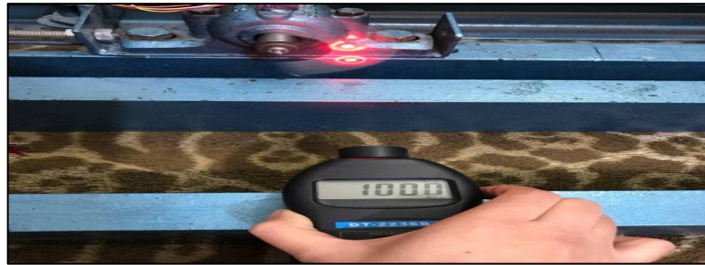
Figure 3: Method of speed measurement
