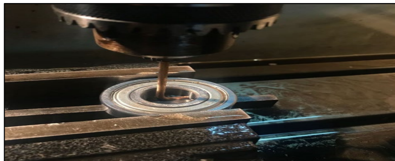
Figure 4: Inner race fault simulation method
