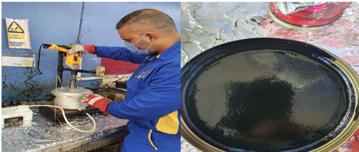
Plate 2: Preparation of asphalt binder modified with (LDPE)
