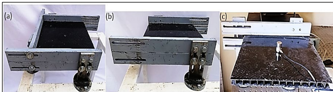
Figure 5: Carbon fiber sandwich specimen under various boundary conditions: (a) Three edges simply supported and one edge free, (b) Two opposite edges simply supported and the remaining edges free and (c) Cantilever
