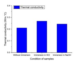
Figure 8: Relation between thermal conductivity and condition of composite.
