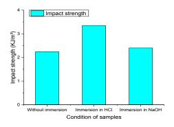
Figure 6: Relation between impact strength and condition of composite.
