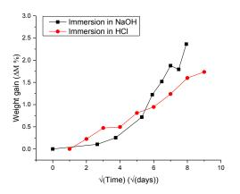
Figure 9: Relation between weight gain vs.  $\sqrt{}$  time (days) of composite
