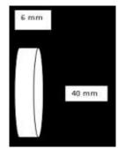
Figure 3: Thermal conductivity test specimen [7]
