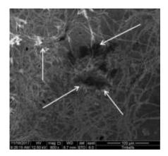
Figure 10: Surface morphology after immersion in NaOH.
