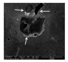
Figure 11: Surface morphology after immersion in HCl.
