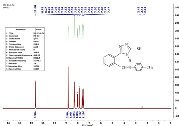
Fig. 3:  $^1\text{H-NMR}$  spectrum of compound (5b) is shown
