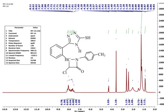
Fig. 4: <sup>1</sup>H-NMR spectrum of compound (6b) is shown
