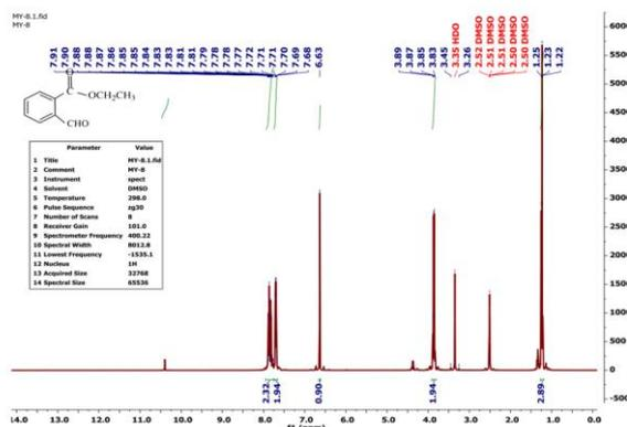
Fig. 1:  $^1\text{H-NMR}$  spectrum of compound (2) is shown
