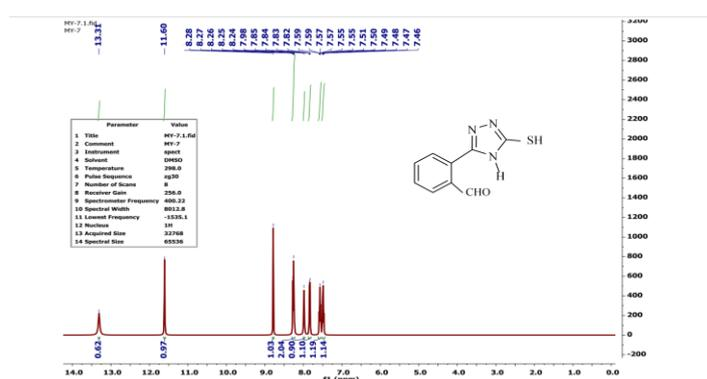
Fig. 2:  $^1\text{H-NMR}$  spectrum of compound (4) is shown
