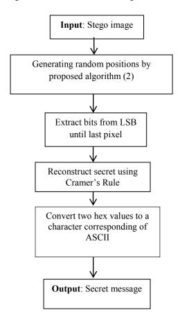
Figure2: Block diagram for extracting text file of proposed method
