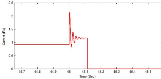
Figure 7: Response of 3-phase current at (L-G) fault
