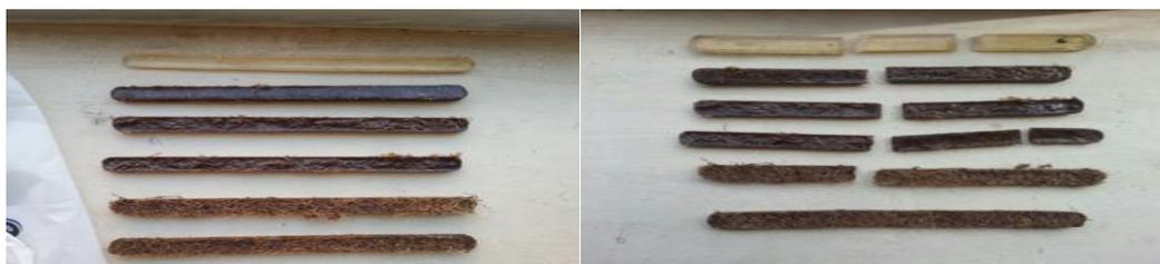
**Figure 4: Flexural Strength experimental specimens before & after test**
