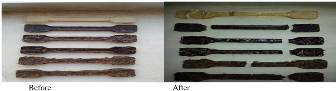
**Figure 2: Tensile test Experimental specimens.**
