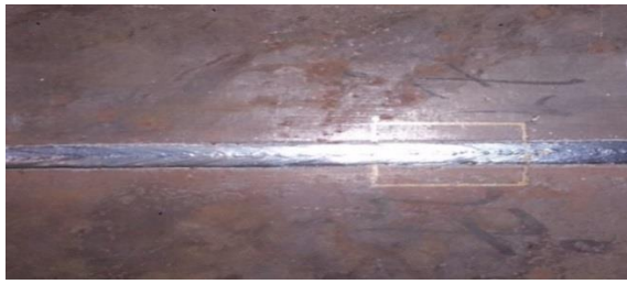
Figure 1: Welded plate sample at input welding factors of run No. 1
