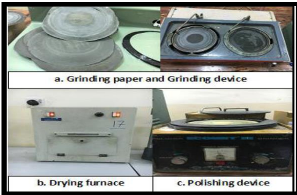
Figure 4: The equipment that used for microscopic imaging
