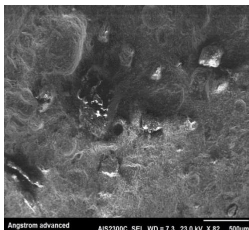
Figure 11: SEM for concrete with micro CaCO 3 .
