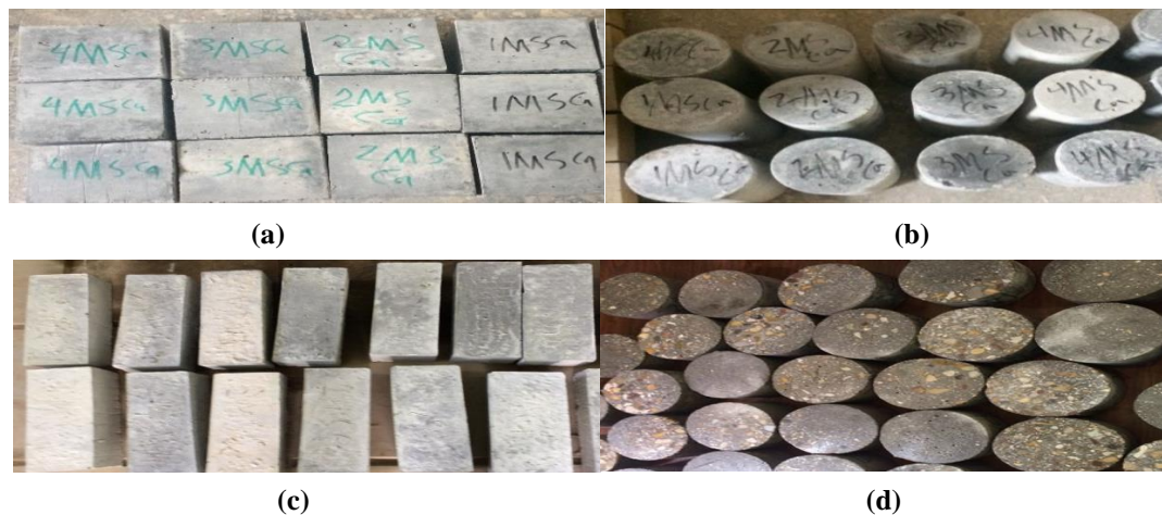
Figure 5: Specimens of test (a) Specimens of compression test. (b) Specimens of split tensile strength test. (c) Specimens of flexural strength test. (d) Specimens of water absorption test.
