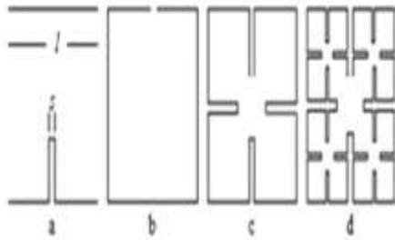
Figure 2: The steps of growth of Minkowski-Like fractal geometry: (a) the generator, (b) the square ring, (c) the 1 st iteration, and (d) the 2 nd iteration[11].
