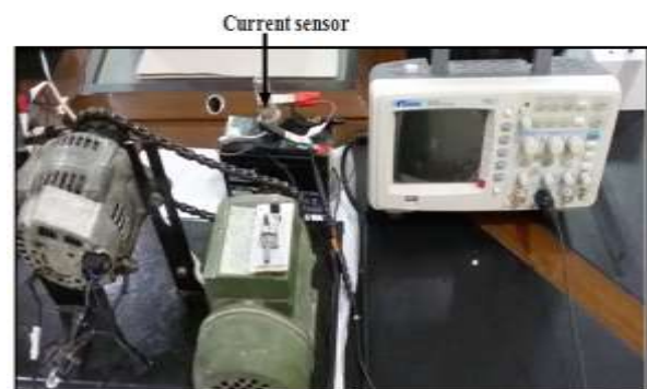
Figure 17: Shows the sensor between the dynamo and battery
