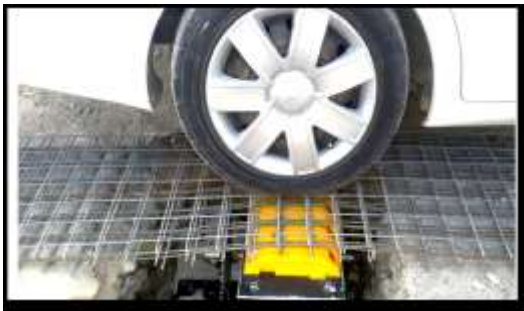
Figure 13: During passage of the back wheel over the speed breaker mechanism.
