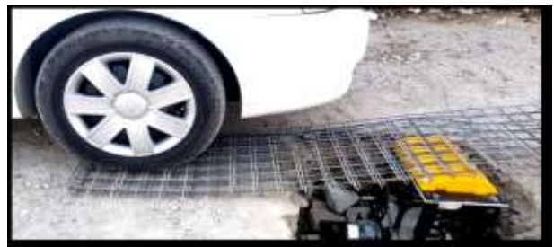
Figure 10: Before passage of the front wheel over the speed breaker mechanism
