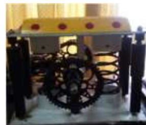
(a)- Front View (b)-Back View Figure 9: Speed breaker mechanism
