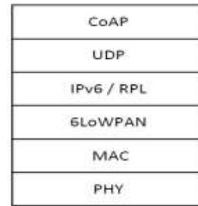
Figure 3: IoT software stack
