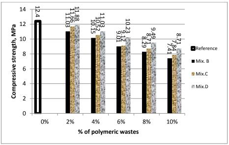
Figure 5: Effect of Polymeric Wastes on the Compressive Strength of Fired Bricks
