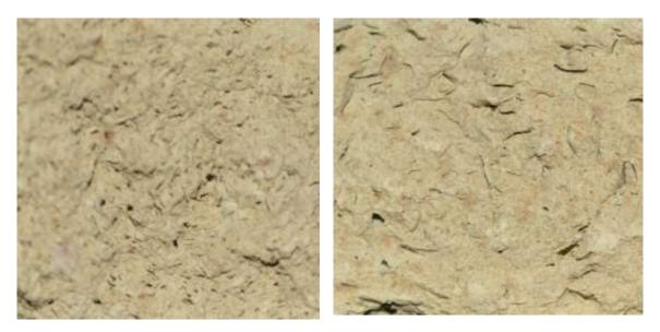
(c) 10wt% Chopped Plastic Addition<br/>(max size 1.18mm)(d) 10wt% Chopped Plastic Addition<br/>(max size 2.36 mm)Figure 3: Surface Texture of Samples with Different Contents and Types of Polymeric Wastes
