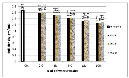
Figure 2: Effect of Polymeric Wastes on the Bulk Density of Fired Bricks
