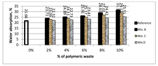
Figure 4: Effect of Polymeric Wastes on the Water Absorption of Fired Bricks
