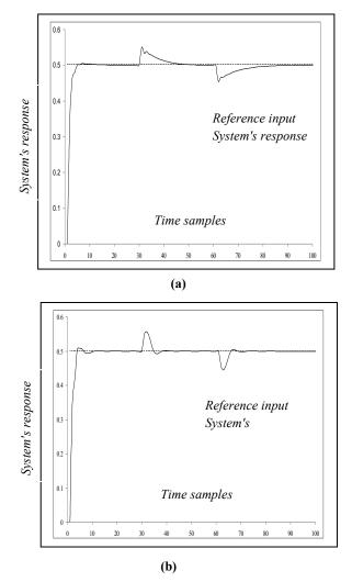
Figure 6: Disturbance rejection tests for (a) Plant 1 (b) Plant 2
