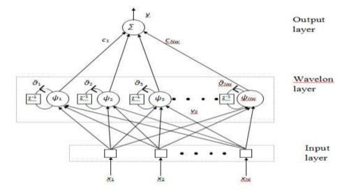
Figure 1: Structure of the SRWNN controller
